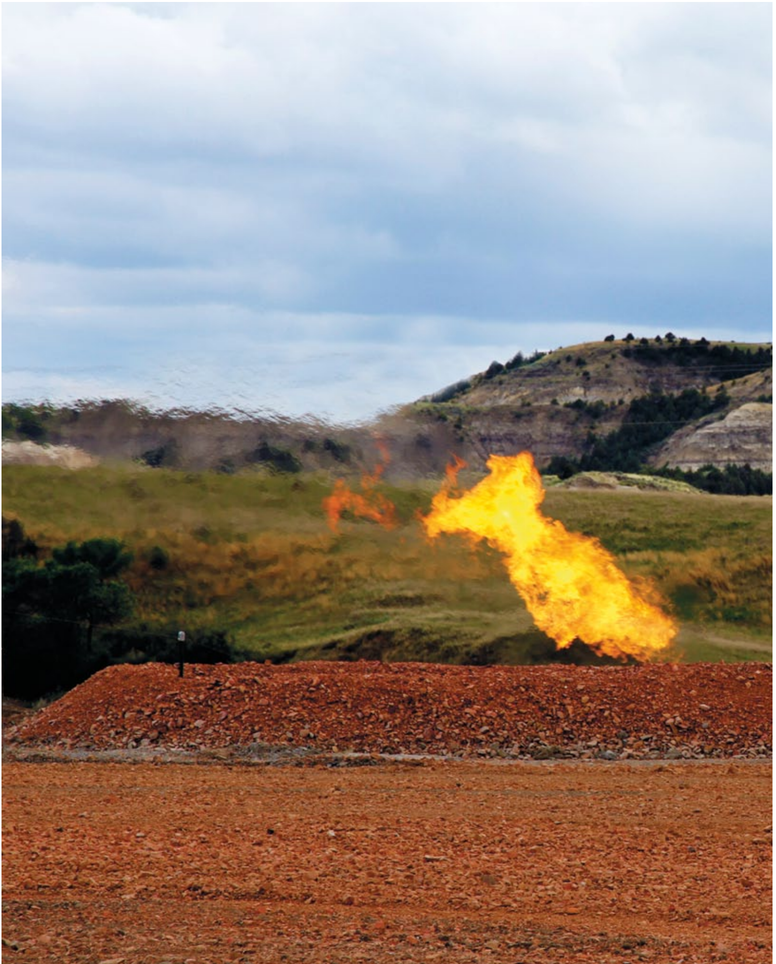
A gas flare at a Bakken oil well in North Dakota. About one-third of gas produced at Bakken oil wells is currently flared. iStock ©mellypage
