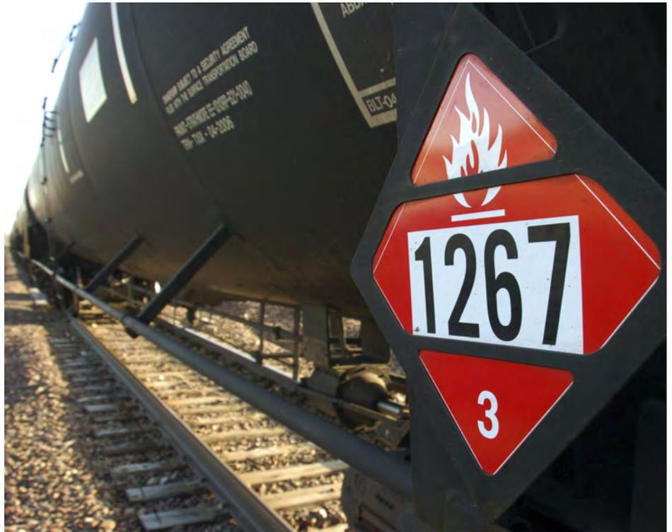
A warning placard on a tank car carrying crude oil is seen on a train idled on the tracks near a crude loading terminal in Trenton, N.D. on Nov. 6, 2013. The number 1267 denotes that the contents of the tank are Petroleum Crude Oil. (©AP Photo/Matthew Brown)
